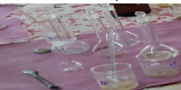
Fig. 14: Specific Gravity Test
